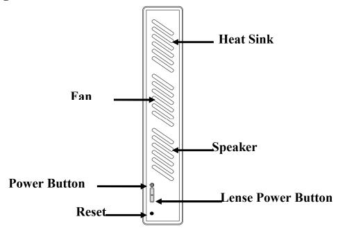
Push and hold the power button for three seconds. Release the power button when the projector begins to project an image
